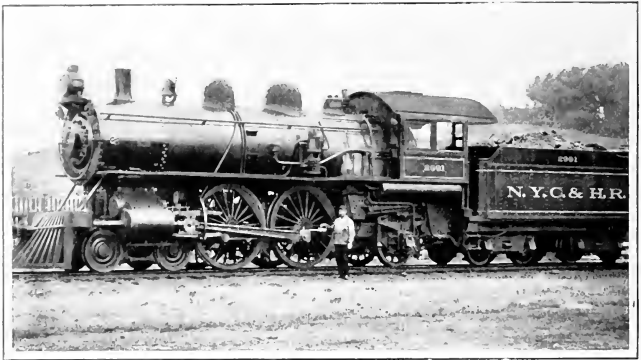
Type of Passenger Locomotive Used on an American Railroad—Weight Eighty-eight Tons (without tender).
